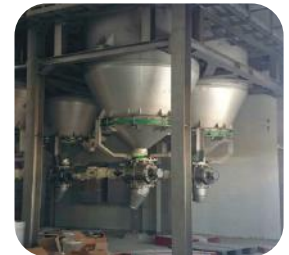
SS304 Hygienic Platform for 50 Ton Silos
