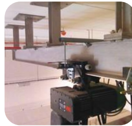
SS304 Hoist Beams with Hygienic Design
