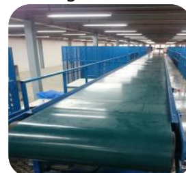
40m Long Belt Conveyor with Single Motor Drive
