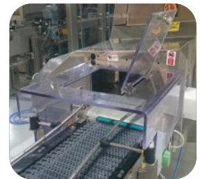
Machine Safety Covers in Polycarbonate
