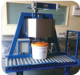
Pneumatic Lid Pressing Machine for Grease Buckets
